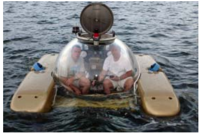
The Triton 1000 has a transparent spherical acrylic passenger compartment
